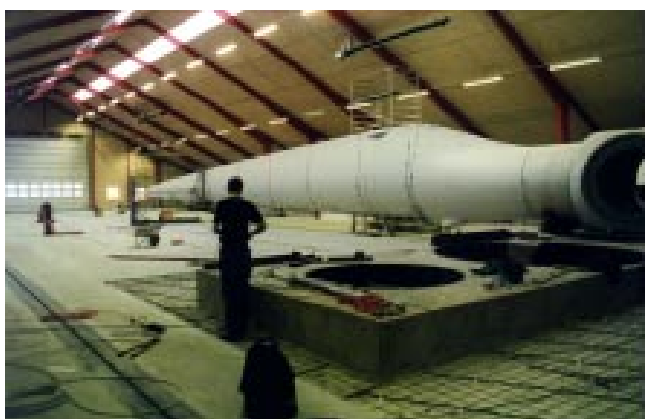
Test of a large blade for a windturbine at Risoe Testcenter in Sparkaer. (Photo: Risø)
